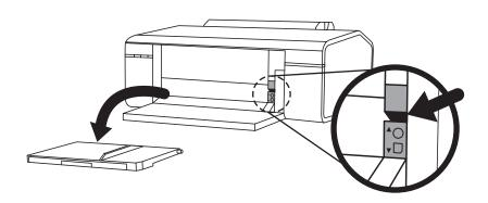
3. Insert Autoloader into printer "disc tray" slots at a 45 degree angle
